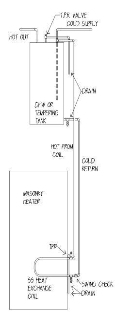
Figure 4. Hot water system -thermosyphon method
