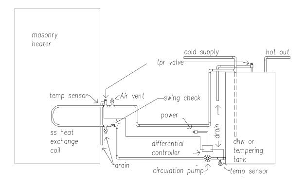
Figure 5. Hot water system - circulation pump method
