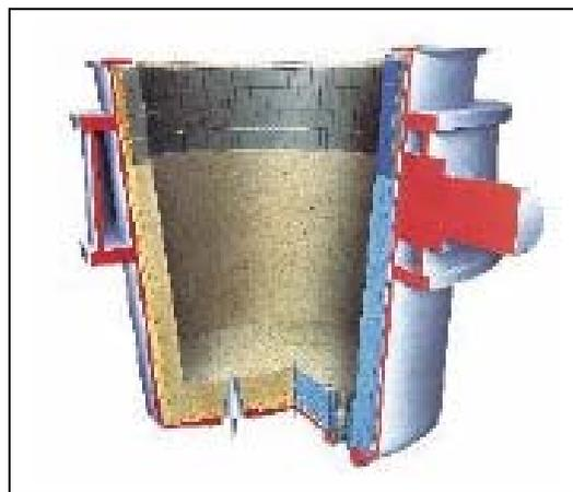
**Figure 9. A Monolithic Lining for Ladle**
