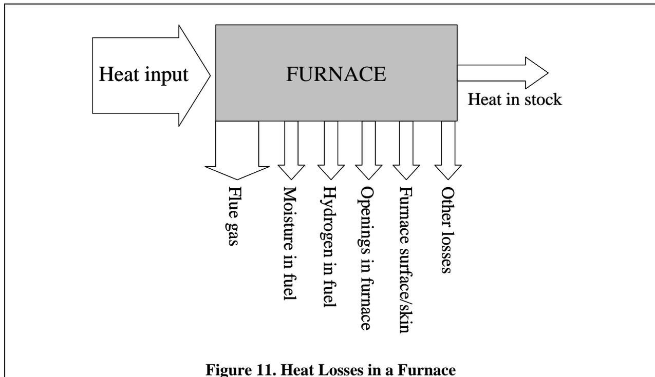
Figure 11. Heat Losses in a Furnace
