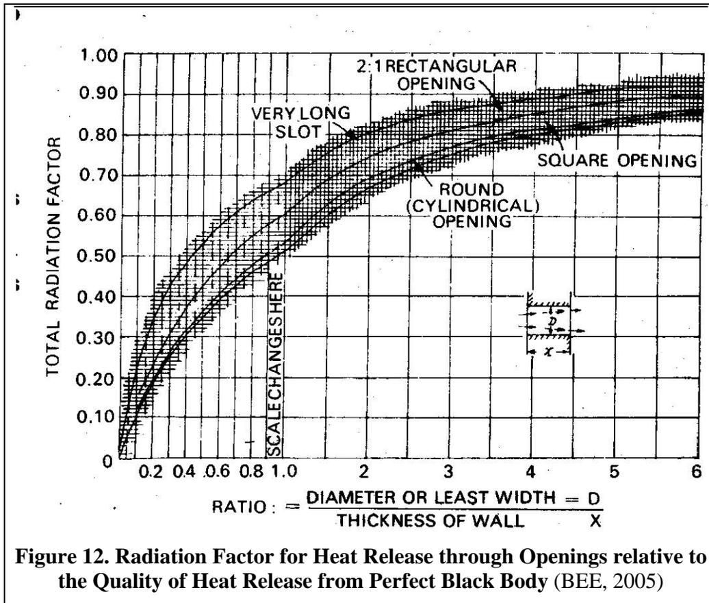
Figure 12. Radiation Factor for Heat Release through Openings relative to the Quality of Heat Release from Perfect Black Body (BEE, 2005)
