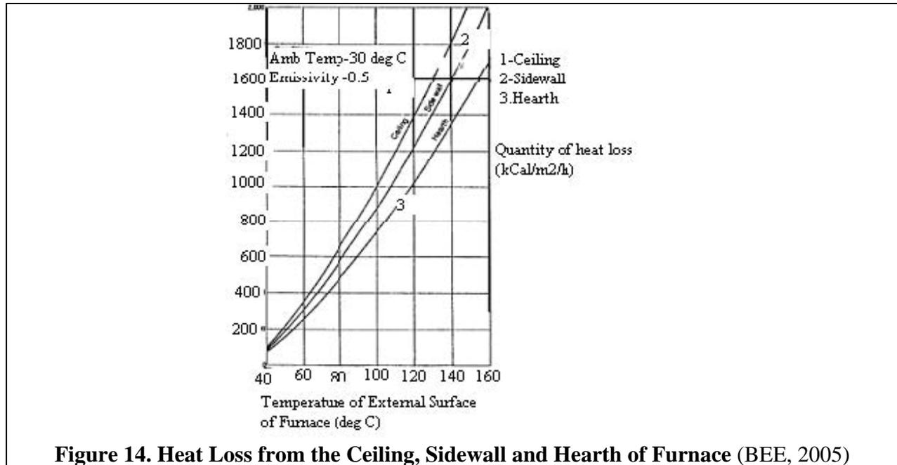
Figure 14. Heat Loss from the Ceiling, Sidewall and Hearth of Furnace (BEE, 2005)
