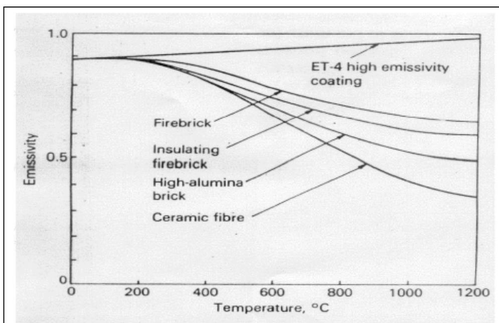
**Figure 10. Emissivity of Refractory Materials at Different Temperatures (BEE, 2005)**
