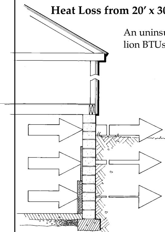
The calculations below assume a 20' x 30' basement with 2' above grade and uniform 8' concrete walls. Doors or windows in poorly insulated homes would generally make the heat loss calculations worse. The calculations are averaged to take into consideration the fact that outside temperatures are warmer below grade.
