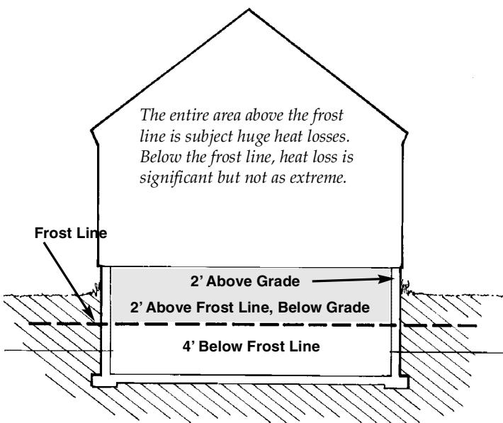
Temperatures below the frost line are relatively stable at 50°. Heat loss is rapid right down to the frost line.
